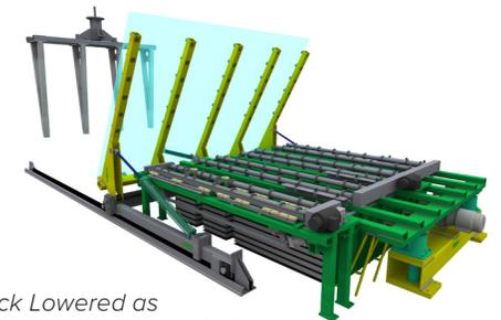
*Storage Rack Lowered as the Tilt Loader Loads the Next Lite*
