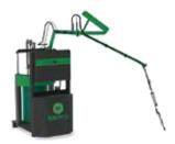
The **Sealing Extruder** uses double-component silicone, polysulphide or polyurethane products, allowing for the final sealing of insulated glass units.
