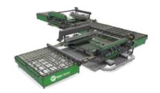
The **Double Edger Line** includes two sets of straight-line glass double edgers and one 90 degree transfer table. It is used to automatically edge and polish the four parallel straight lines of the flat glass.
