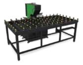
The Sandbelt Glass Grinding Machine is a manual machine with an upper and lower sandbelt designed to grind sharp edges of cut glass before insulated or tempered production. Universal rollers for loading and processing make the machine easy to operate.
