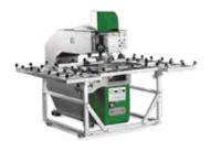
The Glass Drilling Machine is a cold processing machine for easy drilling of holes in glass lites. The machine is equipped with an upper and lower drilling bit and an automatic feeding function for continuous production.
