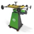
The Rotary Sealing Table has double suction plate and two point rotation (90 degree and 360 degree) to ensure the elements that are optimally secured during the sealing process.
