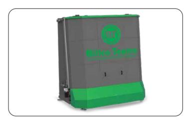
The **Pressing Unit** features a robust, reinforced frame and utilizes a hydraulic or servo-driven front panel system, ensuring consistent and high-quality production. By applying pressure from four distinct points, it delivers precise and reliable insulated glass units.
