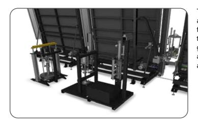
The Servo Motor Control Hydraulic Pump System allows for automatic adjustment of both material flow rate and dosage unit, ensuring precise control throughout the sealing process. This advanced feature guarantees a stable, consistent, and highly accurate automatic glass sealing solution, optimized for reliable and efficient production.
