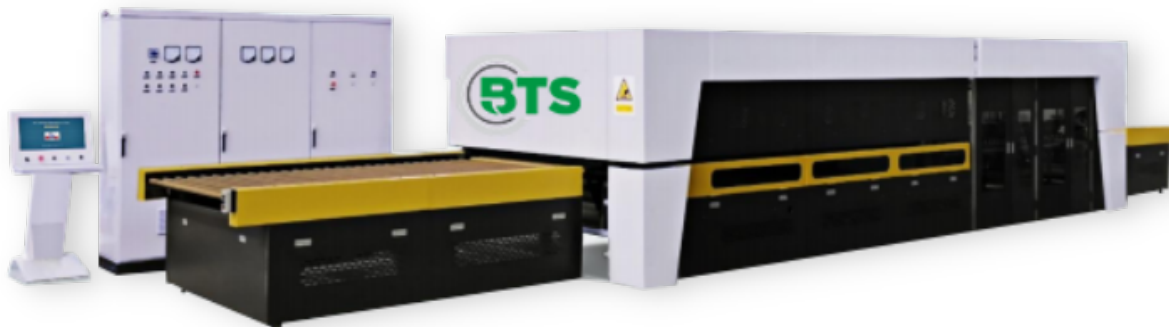
Billco Tempering Systems Convection Furnace
