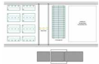
Storage System (Reduced space used by racks 11 - 28. Space increased by 30%.)
