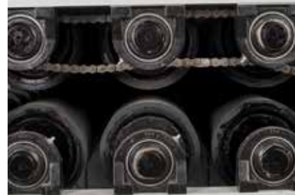
Rollers Progressively Press Units
