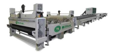
The Lami-Pro is a customizable laminating assembly line built for producing high-quality laminated glass. It is designed to clean the glass, assemble the components, heat, and pre-press the laminated unit before autoclaving.
