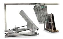
The Crane Loading System is a comprehensive solution for storing, organizing, and loading glass onto the cutting table. This fully automated system retrieves and loads single sheets of glass without operator intervention and can include options for fixed racks and automated compact drawer storage.
