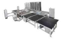
The Remnant Storage Solution automatically identifies, reclaims, stores, and reintroduces remnant lites to the cutting table. This system enhances cutting yield, minimizes unnecessary handling, and eliminates operator error, while effectively removing carts full of glass that often go unused.
