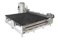
The **Dual Head Ultra Series** is a high-production system designed for high-volume insulating glass production. This machine cuts both lites of glass simultaneously, facilitating easier racking and eliminating wait time for the second lite.
