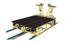
The Automatic Free Fall System retrieves glass from packs and free falls it onto the air float table below. From there, the glass is squared and conveyed to the cutting table for processing.
