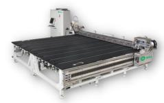
The Dual Head Ultra Series is a high production system specifically designed for large volume insulating glass producers. This machine will cut both lites of glass for a window at the same time, permitting ease of glass racking and eliminating the wait for the second lite.
