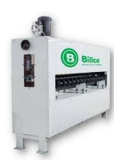
The Cold Roll Press rapidly and uniformly compresses the primary sealing of an insulating glass unit to assure proper "wet-out" and bonding of the spacer sealant to the glass. The Cold Roll Press is offered in both an 84" and 96" working width.
