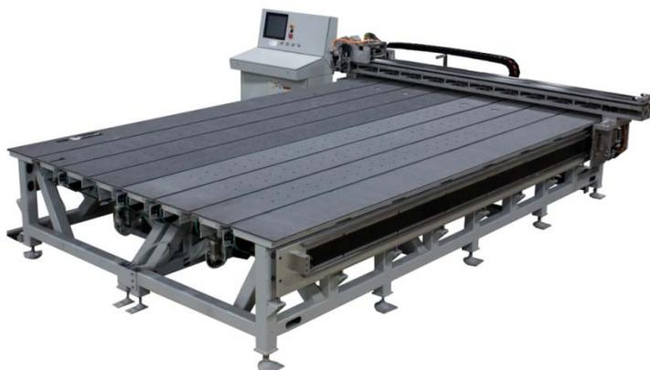
The cutting machine shown above, is typical of the high speed, CNC / XYZ-Contour glass cutting machines, equipped with both scoring and deletion heads that are in use today.
